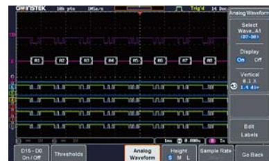
Display analog waveform converted from digital signal
